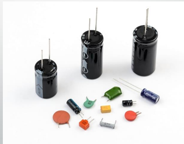
Fixed capacitors: (a) polyester capacitor, (b) ceramic capacitor, (c) electrolytic capacitor.
