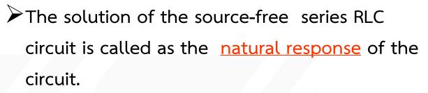
The circuit is <u>excited</u> by the energy initially stored in the capacitor and inductor.
