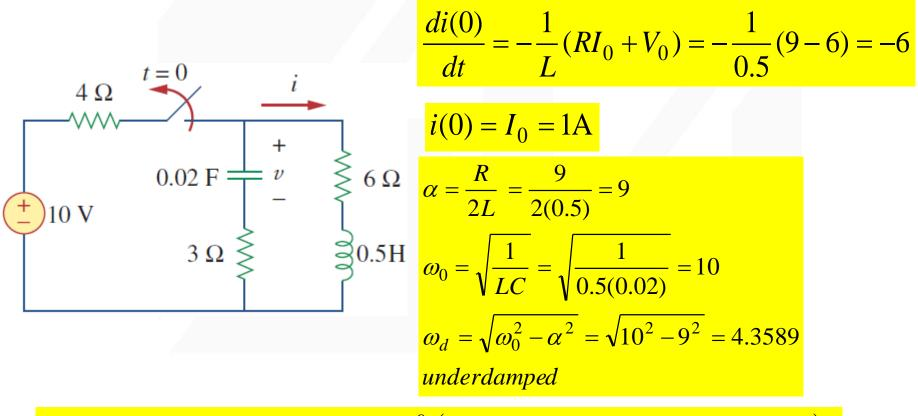
$i(t) = e^{-\alpha t} \left(A\cos\omega_d t + B\sin\omega_d t\right) = e^{-9t} \left(1\cos(4.3589t) + 0.6882\sin(4.3589t)\right) A$
