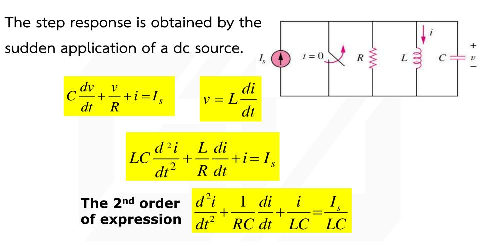
It has the same form as the equation for source-free parallel RLC circuit.
