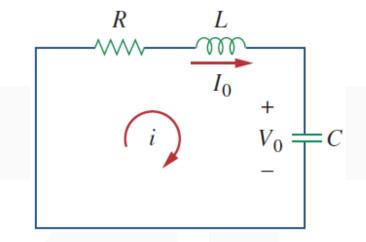
For Capacitor:  $v(0) = v(0^+) = v(0^-) = V_0$ For Inductor:  $i(0) = i(0^+) = i(0^-) = I_0$
